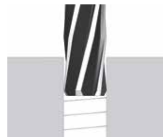
Hole shows chatter or retention marks
