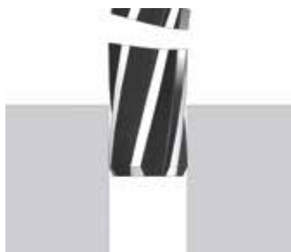
Reamer jams and breaks
