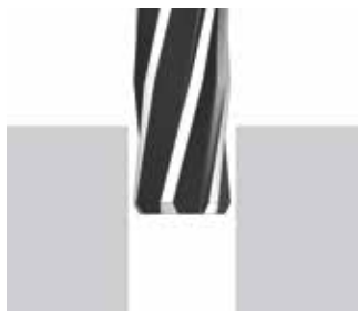
Bore becomes too large
