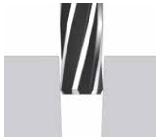
Conical bore (entry too large)
