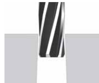
Conical bore (end too large)
